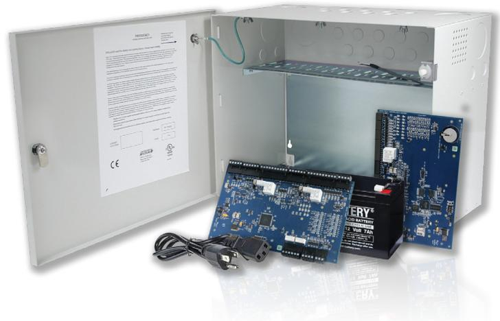
The PRO42OUT interfaces provide up to 16, Form C, 30 VDC, 2A relay output controls depending if the board is rack or tile-mounted, power fail and panel tamper when tile mounted. Relays may be used for elevator control, status annunciation and for general facility control, such as door monitoring.
