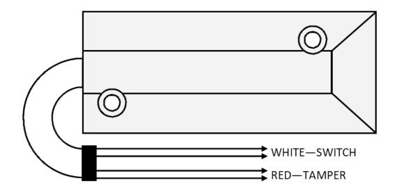
Wire as appropriate for your receiving equipment. Red tamper wires are always a closed circuit. White switch wires will form a closed circuit in presence of the corresponding magnet, opening when the magnet moves away.
